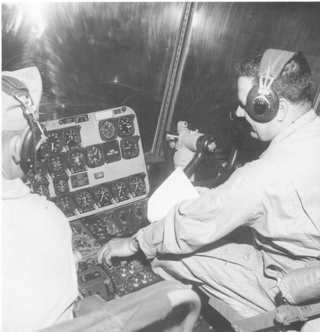
Above, a view of a ZPG-3W cockpit. The N-series airships were the first non-rigid airships to have controls similar to those of an airplane. Below, a ZS2G-1 airship operating at NAS Lakehurst. In the background is a ZPG-2W airborne early warning airship.
